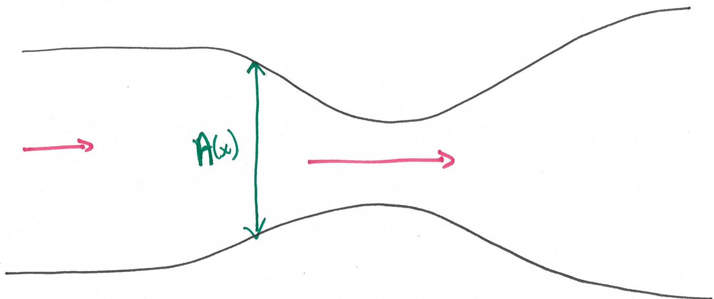
From analysis of Venturi tube, we know flow will accelerate in the neck.
