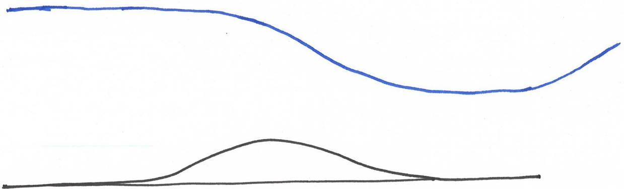
flow becomes asymmetric and develops reduced height  $\Rightarrow$  accelerated flow
