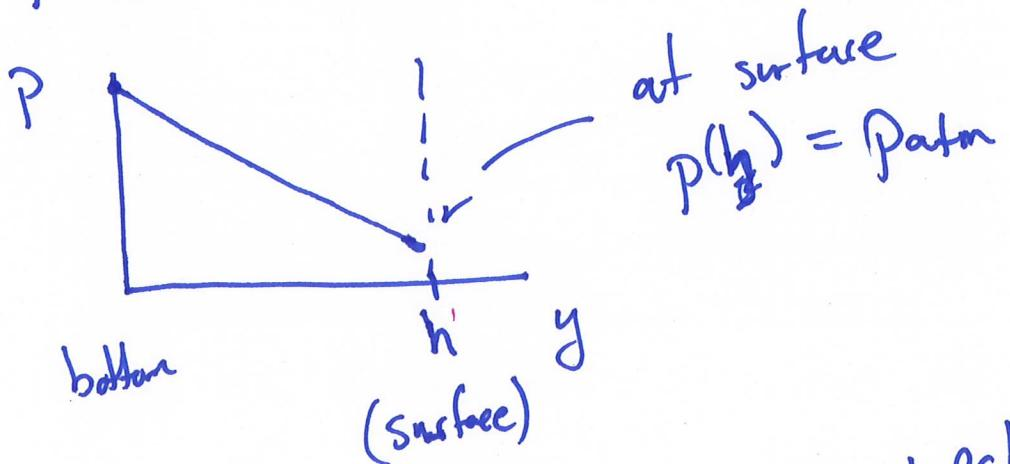
$$P_{\text{atm}} = P_{\text{bottom}} - \rho g h \quad \rightarrow \quad P_{\text{bottom}} = P_{\text{atm}} + \rho g h$$
