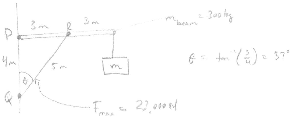
at maximum load, find horizontal component of force at P.
