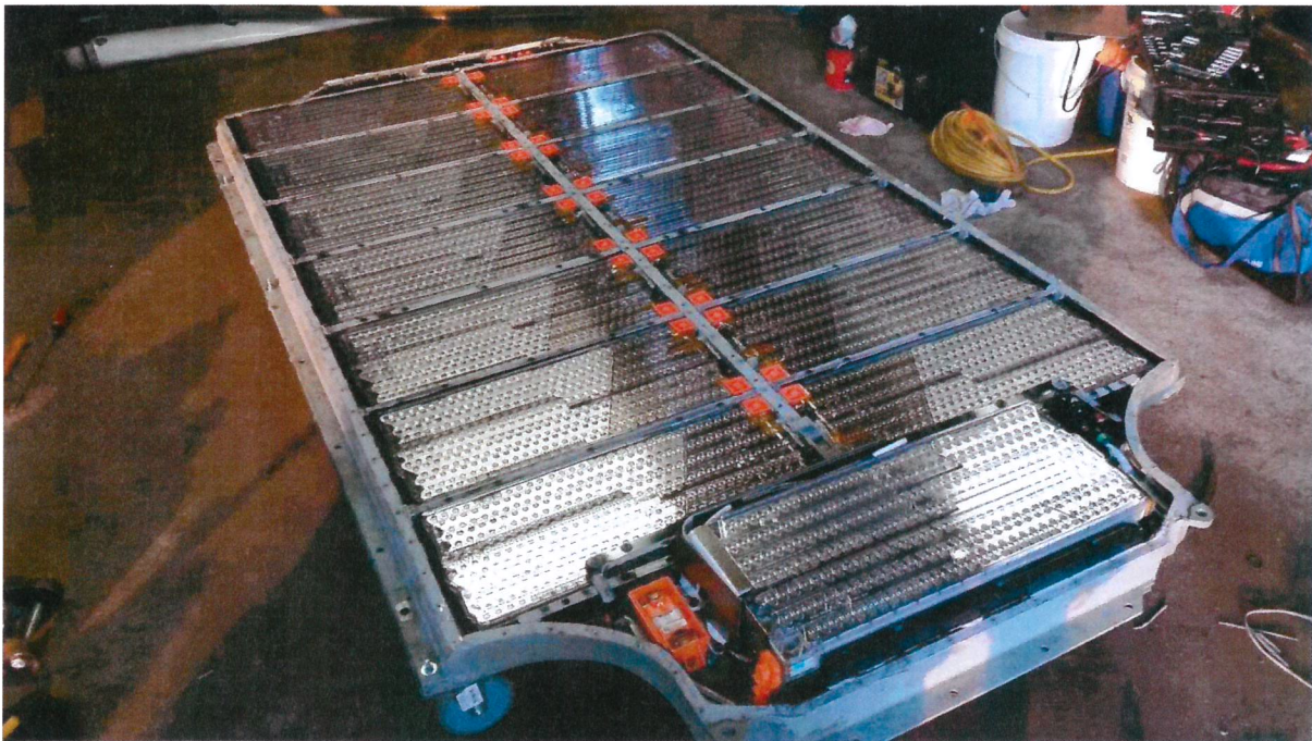
Figure 2. Battery pack inside Tesla Model S, containing 7,104 lithium ion battery cells, to provide the car with 85 kWh of energy at full charge. Figure from: https://insideevs.com/news/323682/rare-look-inside-a-tesla-model-s-battery-pack/ .
