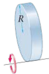
Disk or solid cylinder (axis at rim) I = \frac{3}{2}MR^2
