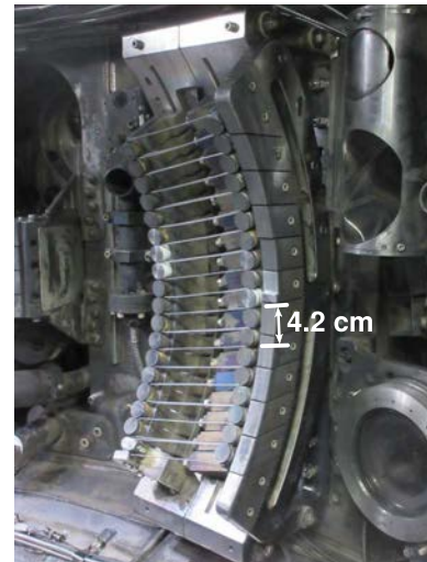
Figure 1. The Shoelace antenna mounted inside the Alcator C-Mod vacuum vessel, as configured in its shifted location for operation in the 2016 experimental campaign.
