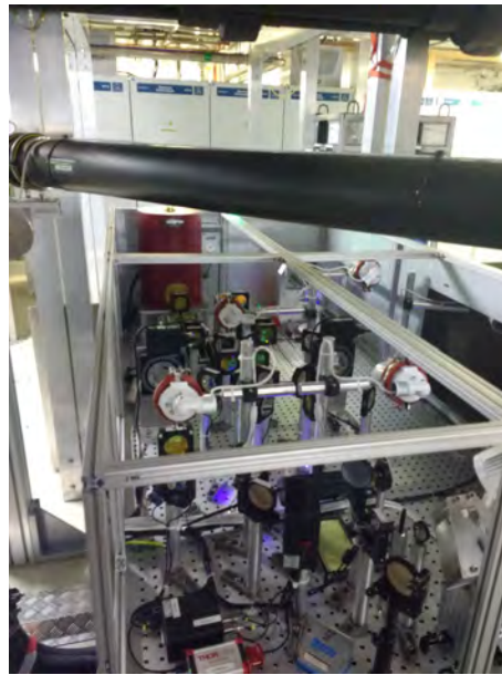
Figure 8: Photo of the receiving table installation. The detector can be seen at the rear-left side of the optics table. The black object above the table is the Thomson scattering beam duct.
