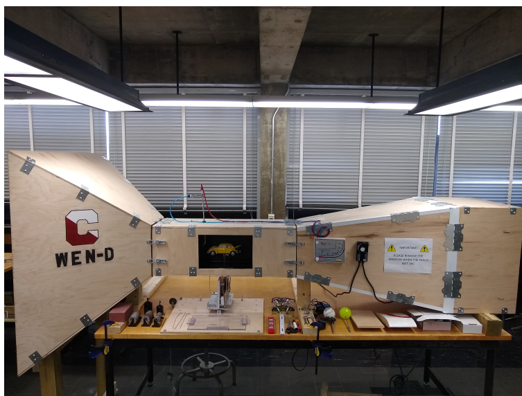
Figure 1: A photograph of the WEN-D wind tunnel at SUNY Cortland (dated May 6, 2021). The fan is located at the far right side of the tunnel, with the test chamber in the middle. The Pitot tube can be seen on the top-left of the test chamber, with the pressure gauge to the right. A two-axis force balance (lift and drag) can be seen below the wind tunnel.
