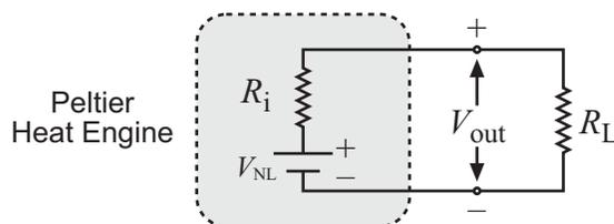
The voltage of the ideal voltage source,  $V_{NL}$ , is called the no-load voltage. For a peltier heat engine  $V_{NL}$  depends only on  $\Delta T$ .
