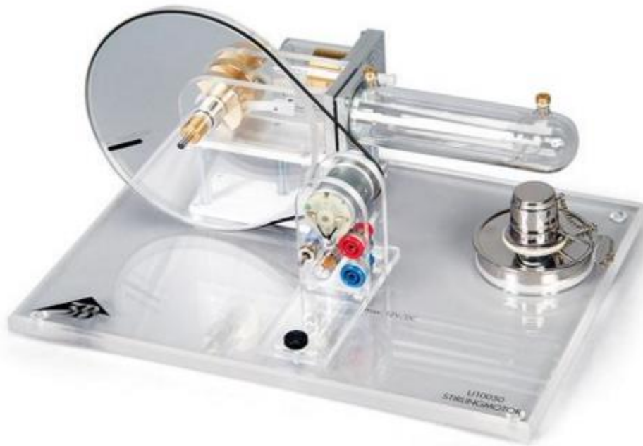
Figure 1 Stirling engine with alcohol lamp heat source and coupled to an electric dynamo. The two small brass circles in the glass tube are in thermal contact with the hot (right) and cold (left) thermal reservoirs [1].
