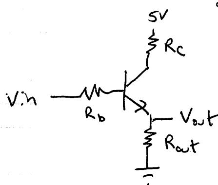
$$\text{loop rule } 5V = V_{RC} + V_{CE} + V_{eot}$$
