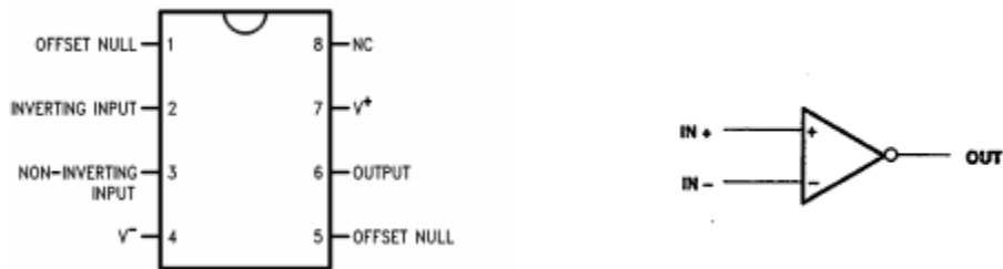
Figure 8.4 LM741 Pin-out diagram and schematic symbol.
