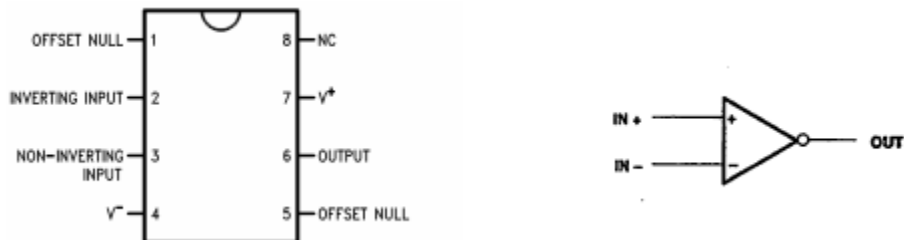
Figure 8.4 LM741 Pin-out diagram and schematic symbol.
