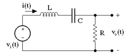
Figure 1: Series LC circuit.
