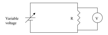
If R is known, then the voltmeter reading is an indication of the current. If the current increases, V increases and vice-versa. If the value of the current is needed, you can calculate it from the V and R.
