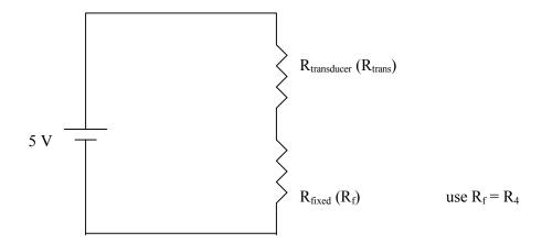
Now place the voltmeter across  $R_f$ . Experiment with changing the value of  $R_{trans}$  by changing the stimulus. Can you detect the changes with your voltmeter? Qualitatively relate the meter reading changes to the stimulus. (For example, does it go up or down with increased light? How much does it change from dark to room light?)
