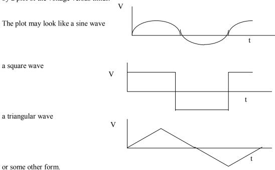
The frequency of the signal is the repetition rate of the regular pattern (frequency is the inverse of the period, which is the time between adjacent peaks). The amplitude of the signal is the maximum voltage of the signal (half the peak-to-peak value). (See the figure below).
