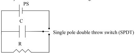
The switch is first thrown so that the power supply is attached to the capacitor. The capacitor is charged until the voltage across it equals that of the source. The switch is thrown the other way so that the power supply is disconnected and the resistor is attached. This gives a path for the capacitor to discharge. Since the rate at which the charge leaves the capacitor is proportional to
