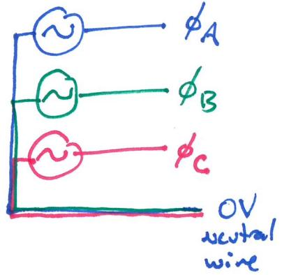
In many situations the returning current for  $\phi_A$  prefers to run on  $\phi_B$ 's  $\phi_C$  so little current flows on the neutral wire. In fact when the loads that  $\phi_A$ ,  $\phi_B$ , and  $\phi_C$  are balanced (definition will follow later) no current flows on the neutral wire.
