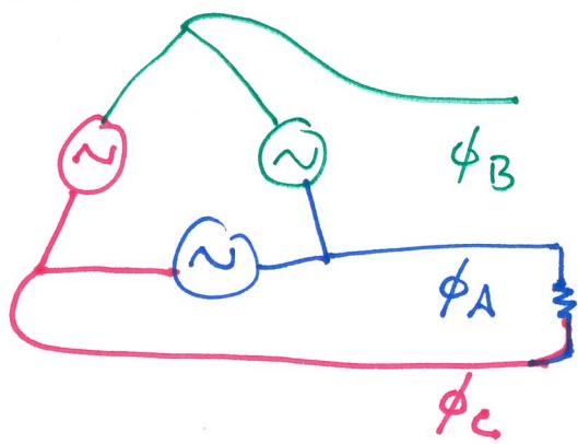
here the resistor is connected to  $\phi_A \setminus \phi_C$  w/ the voltage  $\phi_A - \phi_C$  across it. This is the voltage provided by the Blue power source.
