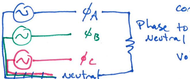
The same load can be connected in 2 ways w/ the WYE topology.
