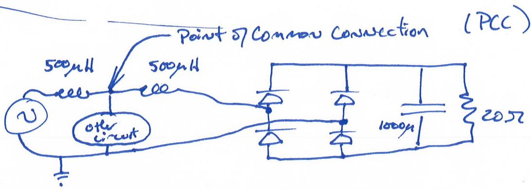
We will observe distortion of the voltage at PCC and measure  $THD_V$  at that location.
