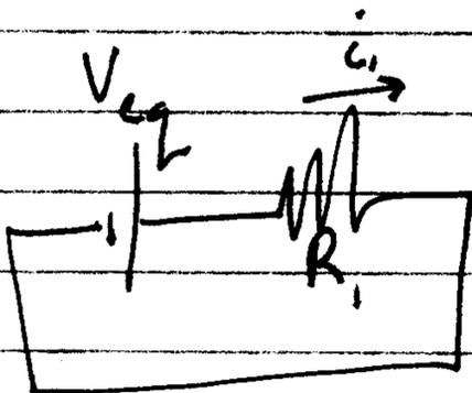
$$V_{eq} = V_1 + V_2 + V_3 = 15V$$
