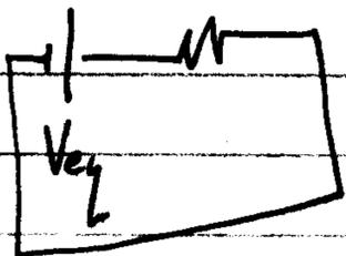
$$V_{eq} = V_S - V_B = 0.8V$$
