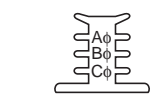
Typical Wiring Diagram Branch connection phasing is determined by circuit breaker selection.
